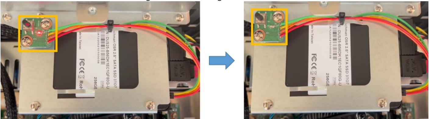
8.2.4 After waiting for 15 minutes, the system will complete the restoration, and the red light will become steady. Once the red light is steady, you can exit the BIOS, restart the system, and Disk C will be restored to its factory state.
