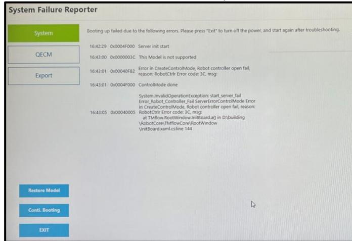
5.16.2.3 Click Restore model. The system will write the corresponding Robot ID into the blank end module and patriot power board base on the robot model last time recorded by the control box. Once the written process is done, the control box will shut down.
