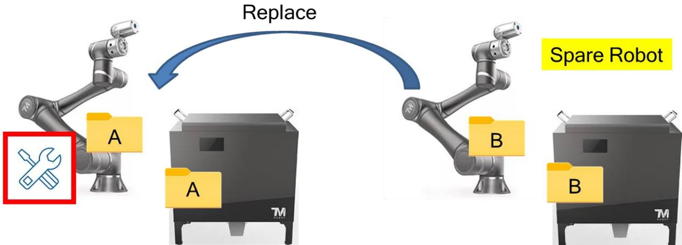
8.3.1 Remove the malfunctioning arm and directly connect the spare arm to the original control box. The calibration data stored in the arm's IO board will overwrite the data in the original control box, so it's crucial to back up the files in the original control box. The software will check whether the data between the arm and control box matches. The following scenarios will explain the handling when the arm firmware (FW) does not match the control box HMI.
