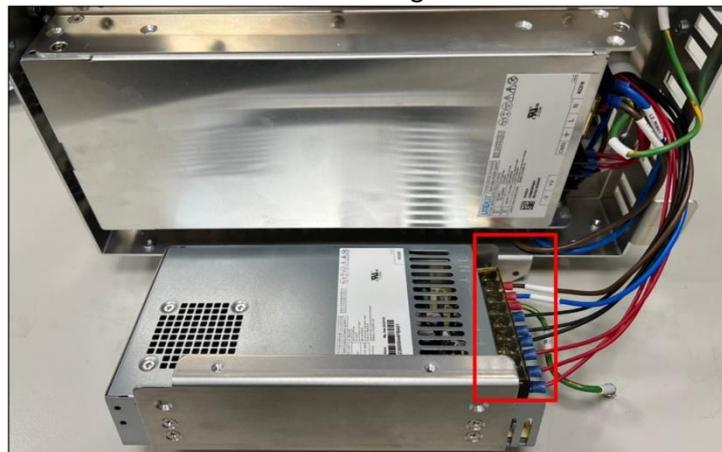
6.11.5 Refer to the diagram below to remove the six bracket securing screws and take out the 24V PSU.
