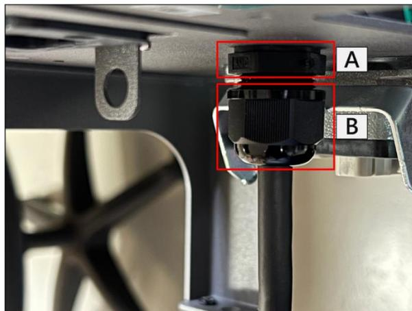
6.6.4 Refer to the diagram to gently bend the Stick connector slightly, and sequentially thread it through the Stick securing nut (Figure A) and the control box (Figure B) to remove the Stick.
