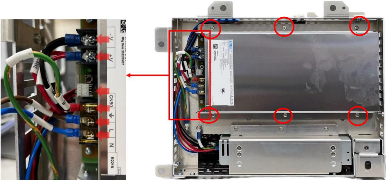
6.10.3 Refer to the diagram below to remove the six securing screws and take out the 48V PSU with the bracket.
