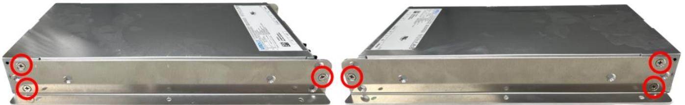
6.10.5 During installation, follow the reverse steps of the above procedure. If cable ties were cut, secure the wires again in the original manner
