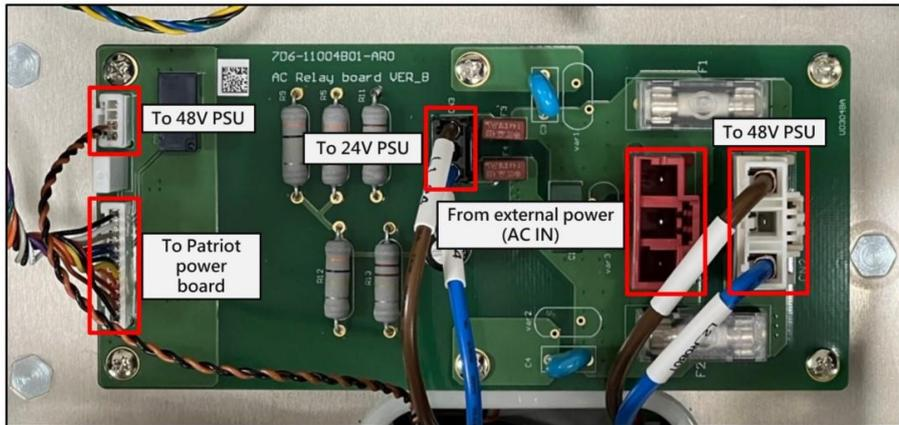
6.5.3 Loosen the 6 screws securing the Relay Board.
