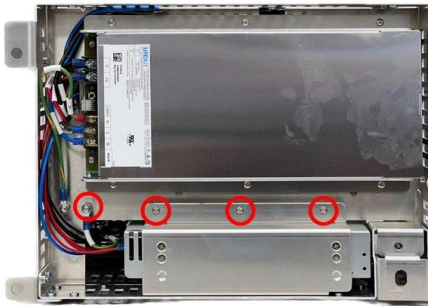
6.11.4 Refer to the diagram below to disconnect the wiring and take out the 24V PSU with the bracket.
