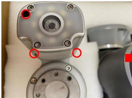
Picture 1 - Remove camera housing screw
