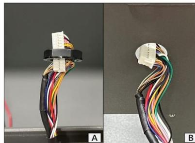
6.6.1 During installation, follow the reverse steps of the above procedure. If cable ties were cut, secure the wires again in the original manner
