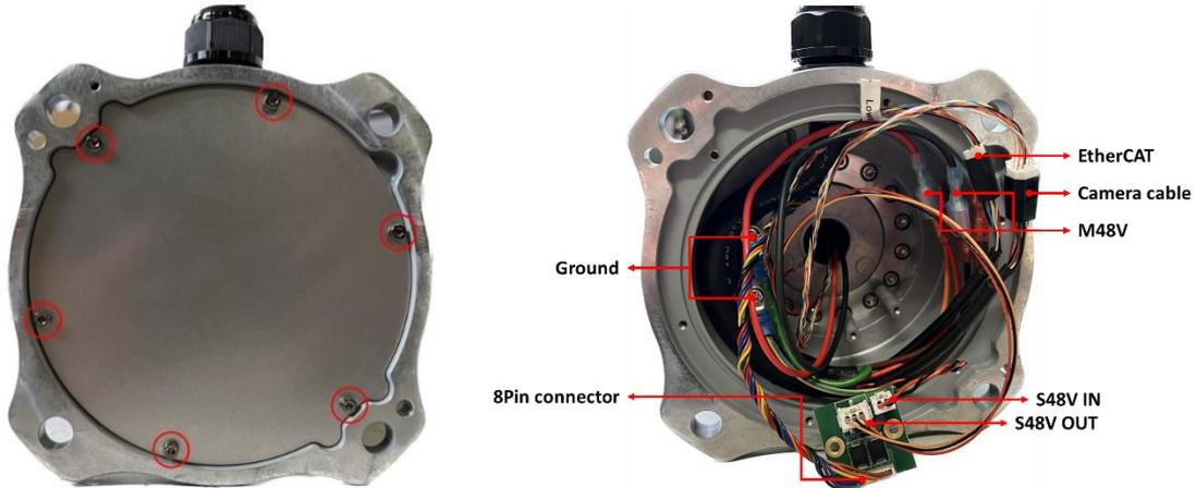
5.6.2 Use wrench to loosen the bottom connector, then carefully pull out the Robot cable.
