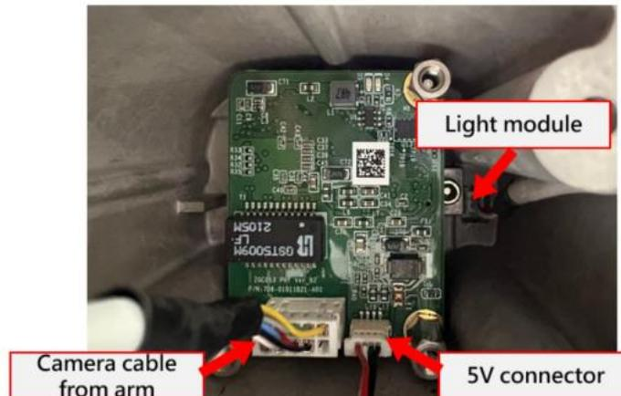
5.14.3 After removing the camera module, take off the three M3L6 screws securing the TRI camera. The torque during assembly is 10 kgf-cm
