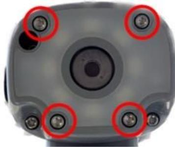
5.13.2 Unplug the power cable of the light source module and remove the light source module, being careful not to let the O-ring fall off.
