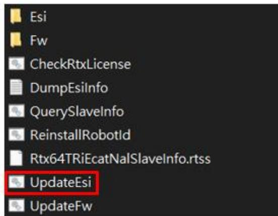
5.16.3.4 UpdateFW: After entering Windows, run the file 'UpdateFW' located in the path: D:\Techman Robot\TM Flow\ModuleRelease. Once the firmware update is complete, completely power off the control box and robot arm. It is recommended to unplug the external power cable after shutting down and then plug it back in to ensure the power is fully turned off before restarting.
