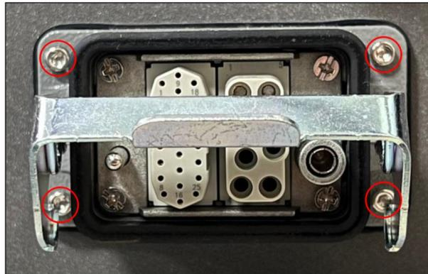
6.7.8 During installation, follow the reverse steps of the above procedure. If cable ties were cut, secure the wires again in the original manner
