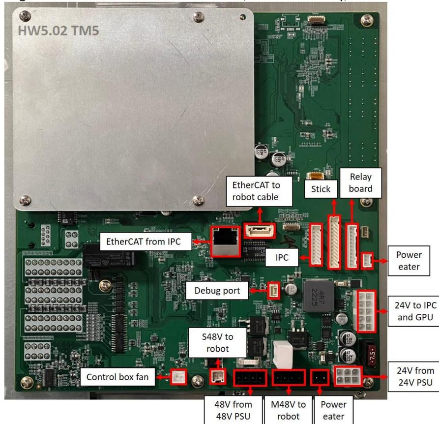
6.4.3 Loosen the 11 screws securing the Patriot Power Board.
