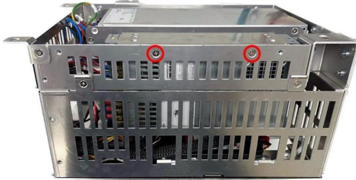
6.11.3 Refer to the diagram below to remove the three securing screws and one grounding wire screw.
