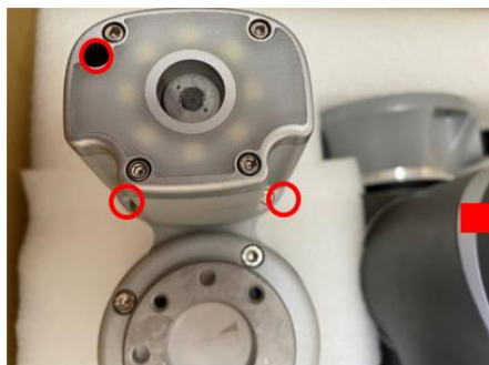
Picture 1 - Remove camera housing screw
