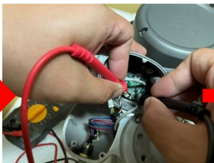
Picture 2 - Measure TRI camera Power
