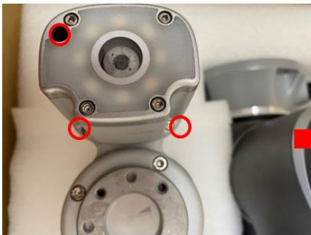
Picture 1 - Remove camera housing screw
