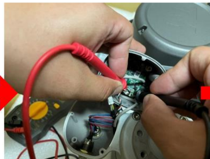
Picture 2 - Measure TRI camera Power
