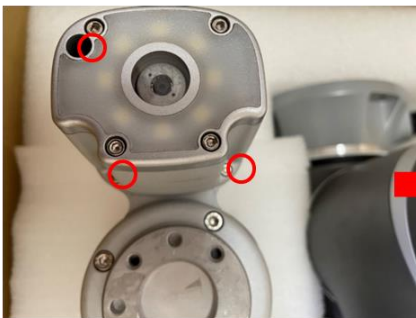
Picture 1 – 移除camera housing螺絲
