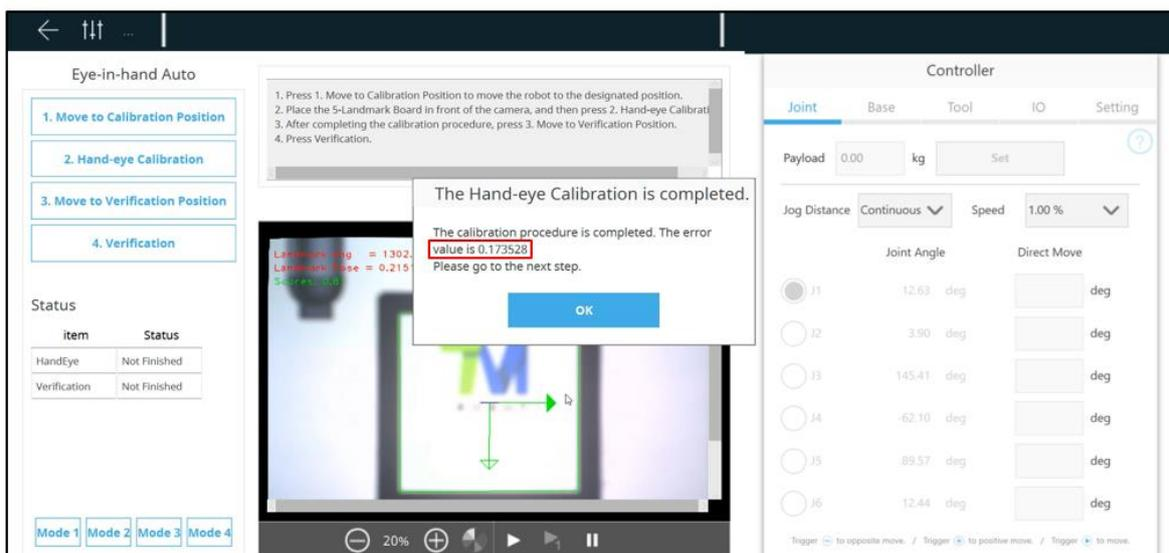
1. Press 'Move to Verification Position' to move the robot to the designated position after completing the hand-eye calibration.
