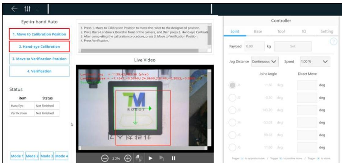
1. Upon completion, if the error value is lower than 0.3, it means the calibration is successful. If the value exceeds 0.3, recalibration is required. At this point, adjust the camera parameters and the surrounding lighting in the field, ensuring that the robot and the platform with the placed landmark remain stable and do not shake.
