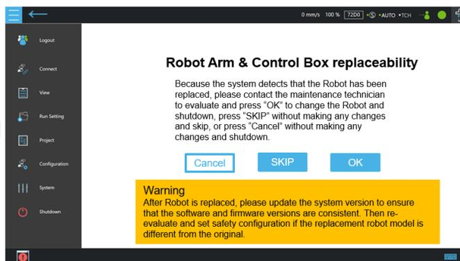
5.16.7 When replacing a new end module or its PCBA, user needs to go to maintenance mode and perform the following steps:
