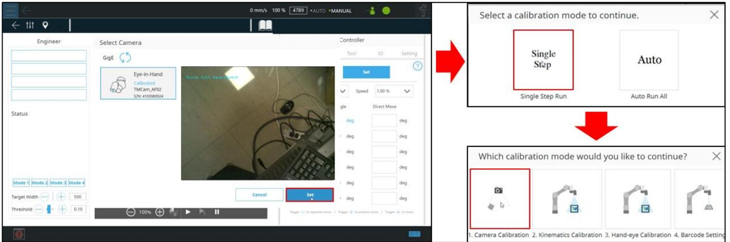
1. Use ① to move the robot to the designated position, then place the **small dice board** and make sure the camera can see the entire dice board as shown in ②
