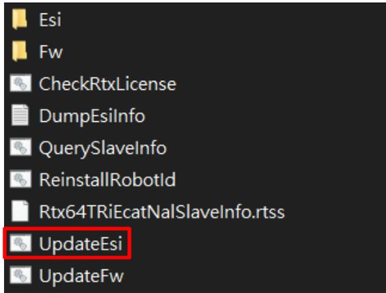
5.16.5 **UpdateFW:** After entering Windows, execute the file "UpdateFW" in the path "D:\Techman Robot\TM Flow\ModuleRelease". After completion, it is necessary to completely turn off the power to the control box and the robot before restarting. It is recommended to unplug the external power cord after shutdown and then reconnect it before turning the power back on, ensuring a complete power shutdown.
