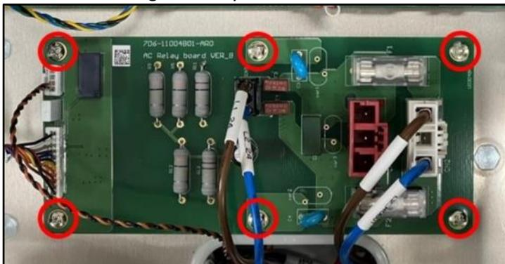
6.5.4 During installation, follow the reverse steps of the above procedure. If cable ties were cut, secure the wires again in the original manner
