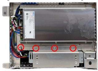
6.11.4 Refer to the diagram below to disconnect the wiring and take out the 24V PSU with the bracket.
