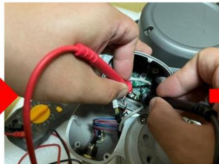
Picture 2 - Measure TRI camera Power
