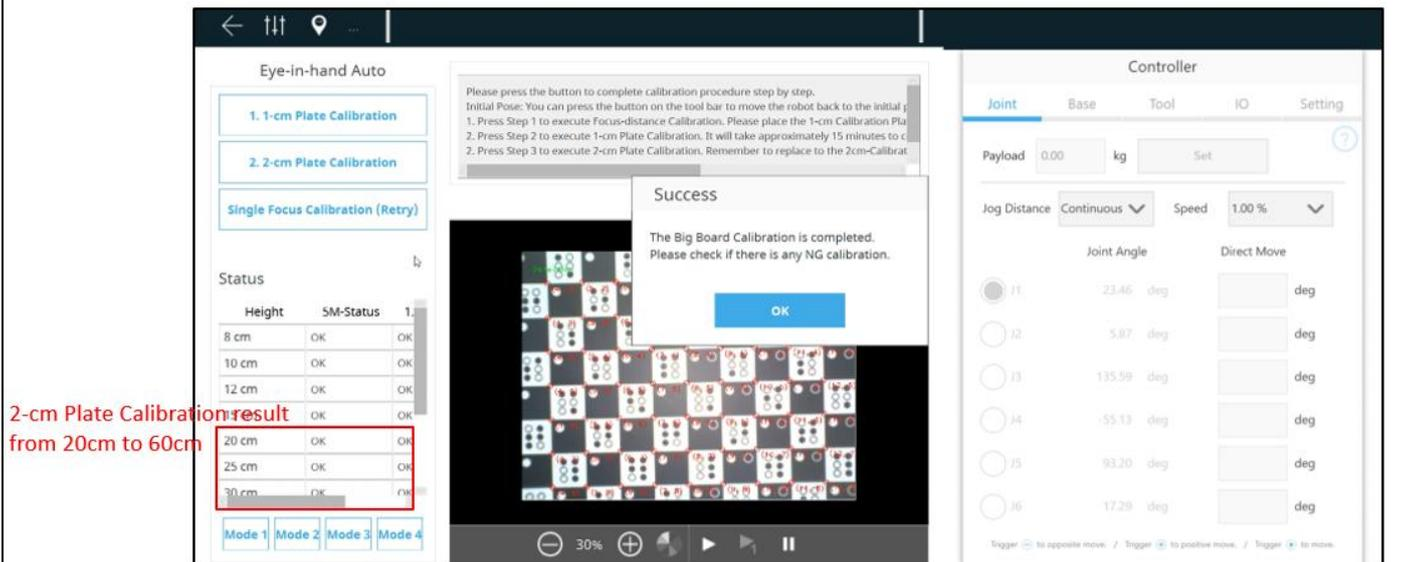
1. If there is any status showing 'not finished' after completing the 2-cm Plate Calibration, use 'Single Focus Calibration' for re-calibrating.
