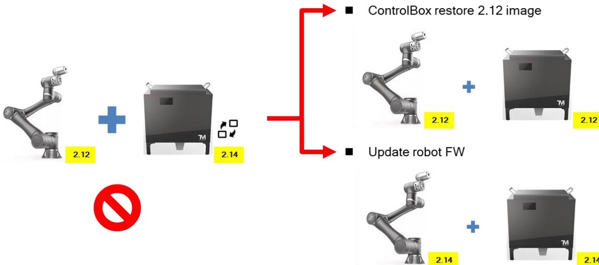
8.3.3 When the arm FW is version 2.14, but the spare control box's HMI version is 2.12, the user can only upgrade the control box's HMI to match the FW. The main reason is that older versions of software or firmware may not recognize the new Joint type.
