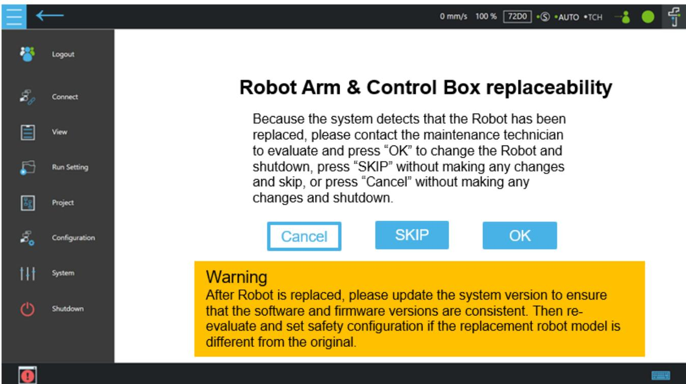
If all the above criteria are met, but the data on the arm side differs from the data on the control box side, switch to this special page after turning on the machine.
