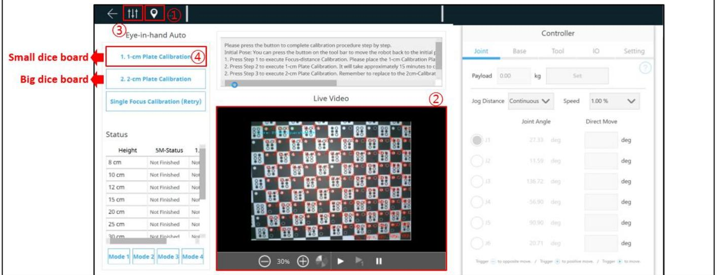
1. Setting up the **big dice board** properly after 1-cm Plate Calibration (small dice board) is completed.
