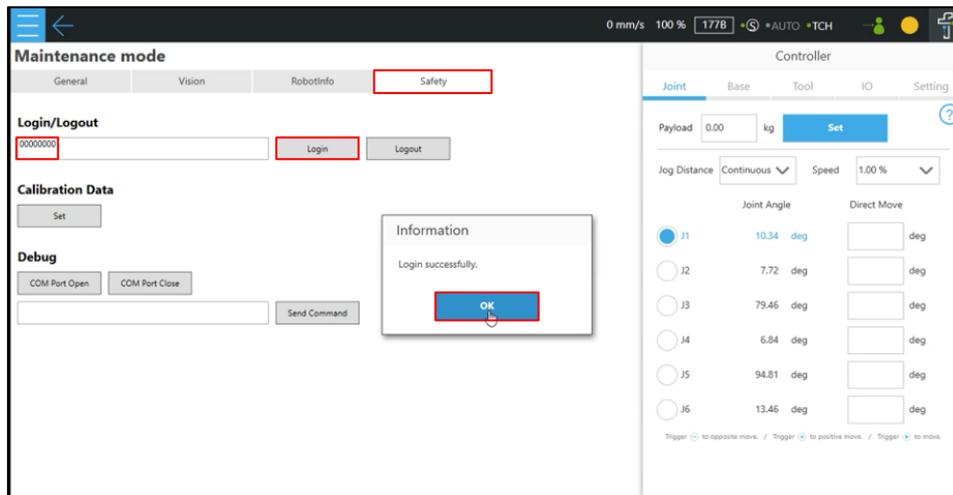
1. Press 'Set' to upload the calibration data from control box to arm
