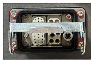
6.7.8 During installation, follow the reverse steps of the above procedure. If cable ties were cut, secure the wires again in the original manner
