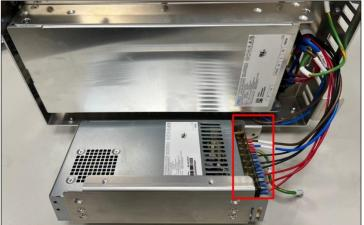
6.11.5 Refer to the diagram below to remove the six bracket securing screws and take out the 24V PSU.
