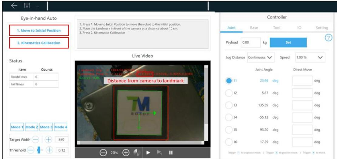
1. Calibration will end upon the successful completion of 40 sets or when failures reach 15 sets.
