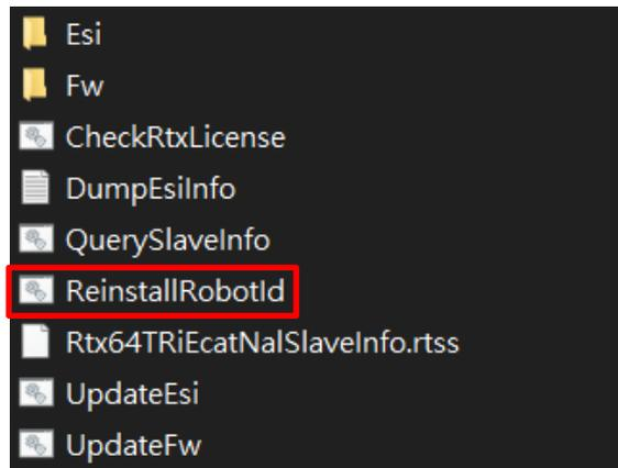
5.16.4 **UpdateEsi:** After entering Windows, execute the file "UpdateEsi" in the path "D:\Techman Robot\TM Flow\ModuleRelease". After completion, it is necessary to completely turn off the power to the control box and the robot before restarting. It is recommended to unplug the external power cord after shutdown and then reconnect it before turning the power back on, ensuring a complete power shutdown.
