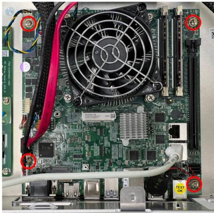
6.3.4 During installation, follow the reverse steps of the above procedure. If cable ties were cut, secure the wires again in the original manner.
