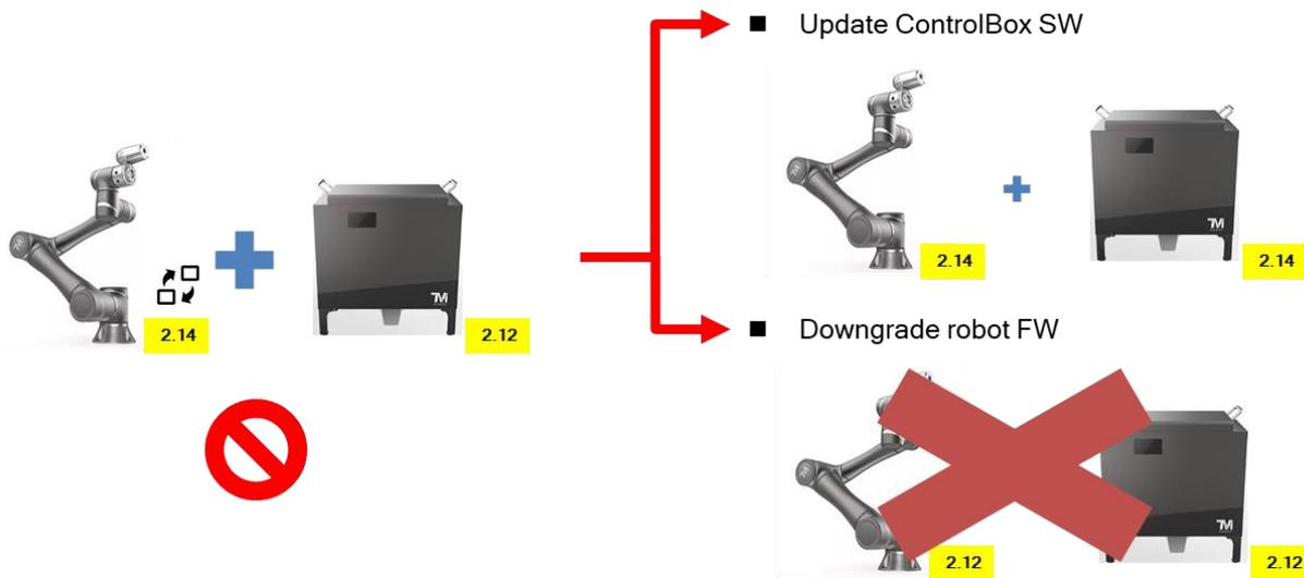
8.3.4 Not every arm and control box can support interchangeability. Exchange can only occur when Arm Model and Control Box Model are mutually compatible. The **Compatibility List** table below summarizes all compatible combinations. Only the Arm model and Control box model appearing simultaneously in the same column of the table can be interchanged.
