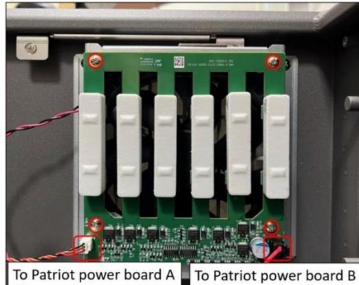
6.9.3 During installation, follow the reverse steps of the above procedure. If cable ties were cut, secure the wires again in the original manner.
