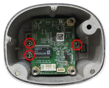
5.14.4 After removing the TRI camera unit (refer to the below picture), replace it directly with a new TRI camera. Do not perform any disassembly or modifications on the components of the unit.
