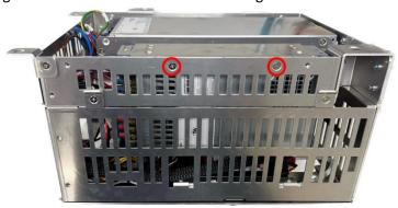
6.11.3 Refer to the diagram below to remove the three securing screws and one grounding wire screw.
