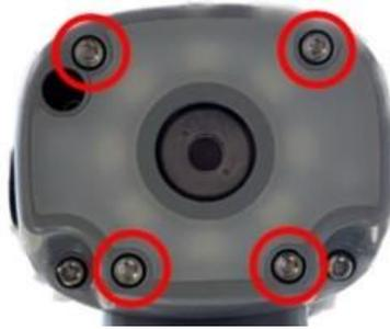
5.13.2 Unplug the power cable of the light source module and remove the light source module, being careful not to let the O-ring fall off.
