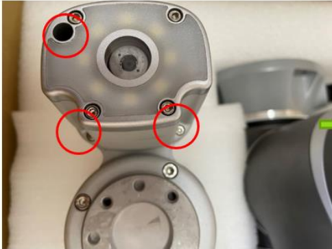
Picture1 Remove camera module screw
