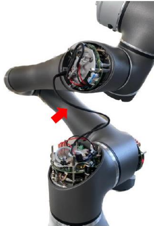
Use additional signal cable or cable dissembled from other joints
